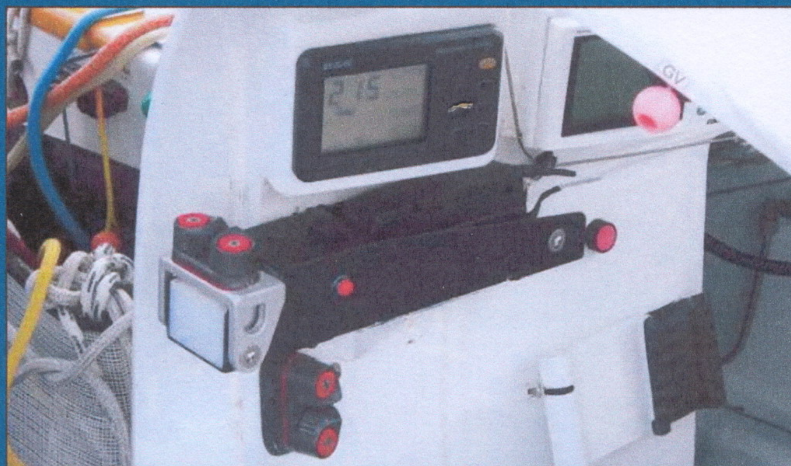
The foresails sheet-release system.
